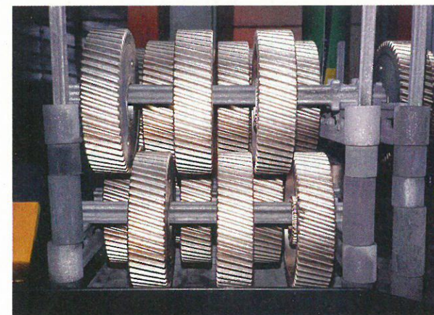
Fig. 4. Example of a dense load of gears
