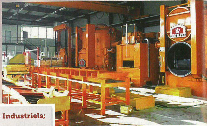
Fig. 6. Example of a flexible vacuum processing cell including oil-quenching furnace
