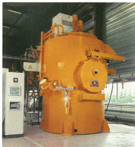
Fig. 7. Oil vacuum furnace type P164TH
